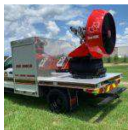
LARGE-FLOW VENTILATOR EASY 4000 TRAILER-MOUNTED 234,430 CFM OPEN AIR
