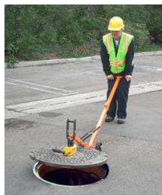
U.S.SAWS MAGNETIC LID LIFTER THREE SIZES FOR WEIGHTS OF 330 – 450 – 660 POUNDS
