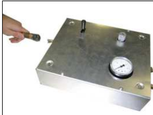
Figure 33. High pressure air source connection.
