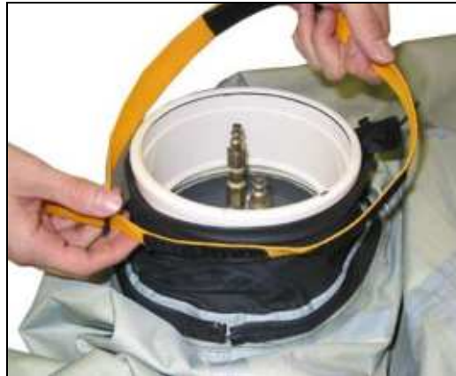
Figure 27. Installing cinching strap.
