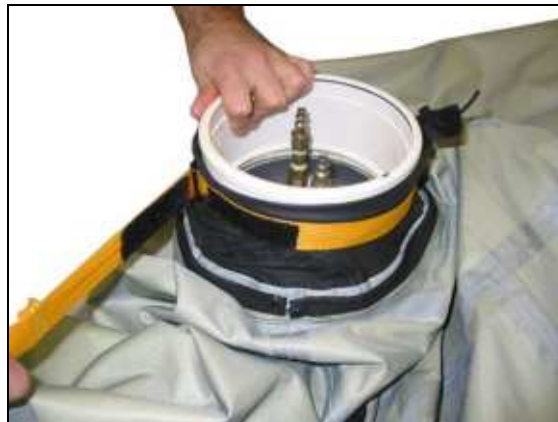
Figure 28. Securing cinching strap.
