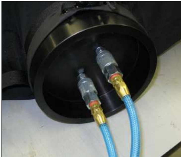
Figure 9. Step i. Suit Leakage Test
