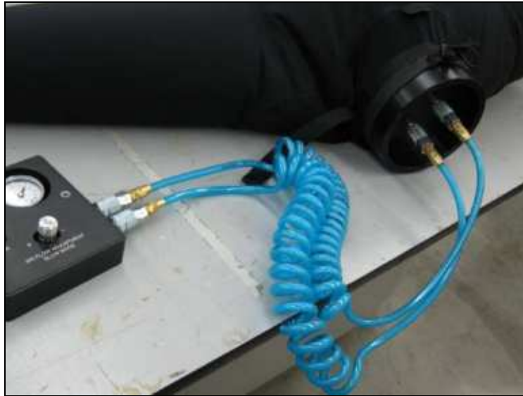
Figure 10. Step j. Suit Leakage Test
