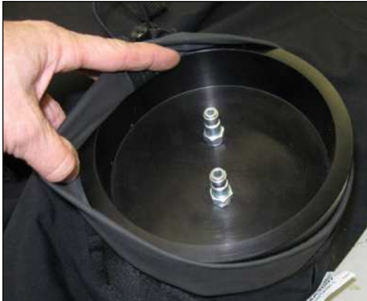
Figure 4. Step d. Suit Leakage Test
