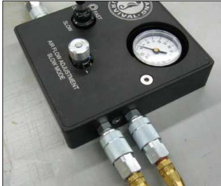
Figure 8. Step h. Suit Leakage Test
