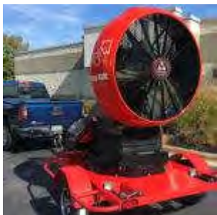
GAS-DRIVEN FAN MT296 56,505 CFM OPEN AIR
